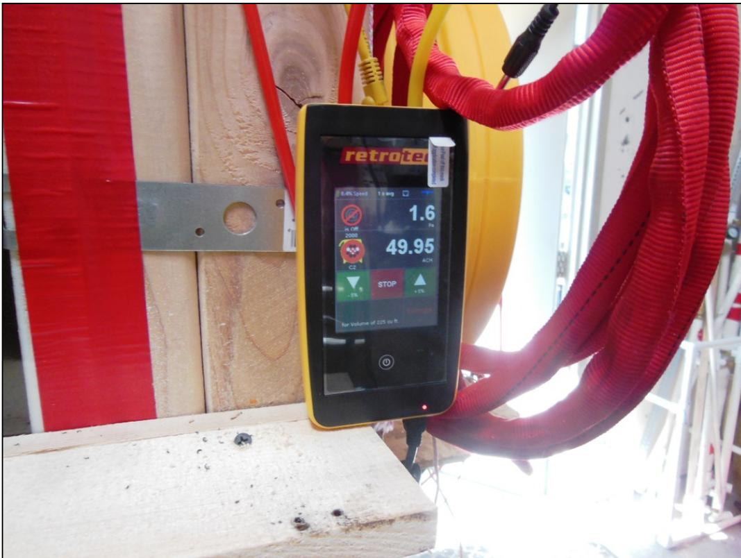
The air exchange rate of 50 ACH was chosen as it represents the likely flows associated with a properly vented ½” rainscreen cavity, based on previous publications <sup>4,5</sup>, accounting for thermal and moisture buoyancy, convection due to thermal gradients, vent occlusion, and wind driven air pressure.
